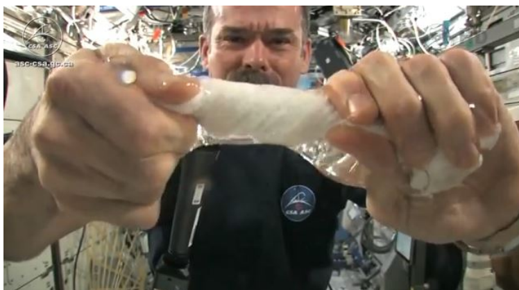
Figure 5.3.2: The Effects of the High Surface Tension of Liquid Water. The Full video can be found at https://www.youtube.com/watch?v=9jB7rOC5kG8 .
