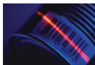
Figure 1.2.4 A Beam of Red Light Emitted by a Helium Neon laser reads a bar code. Originally Helium neon lasers, which emit red light at a wavelength of 632.8 nm, were used to read bar codes. Today, smaller, inexpensive diode lasers are used.
