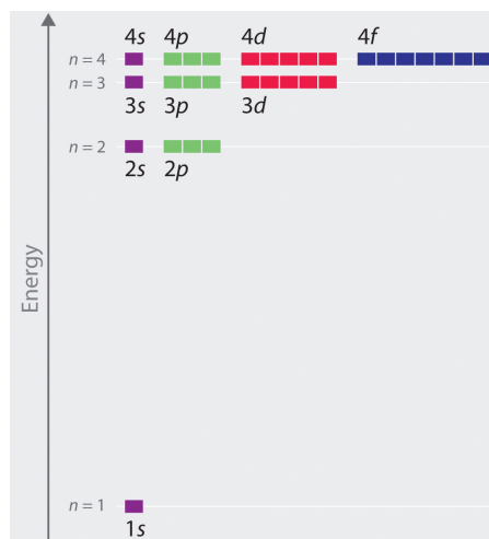
Figure 1.6.6: Orbital Energy Level Diagram for the Hydrogen Atom. Each box corresponds to one orbital. Note that the difference in energy between orbitals decreases rapidly with increasing values of n .
